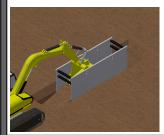
1) EXCAVATE UNTIL SOIL BEGINS TO CRUMBLE BEYOND **DESIRED TRENCH** WIDTH. PLACE SHIELD IN LINE OF **EXCAVATION AND EXCAVATE FROM** WITHIN.
