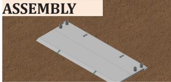
1) REMOVE FROM TRUCK BY LIFTING PANELS WITH 4 POINT LIFT LUGS. ALWAYS USE OSHA APPROVED SLINGS. PLACE ONE SIDEWALL FLAT ON THE GROUND WITH COLLARS FACING UP.
