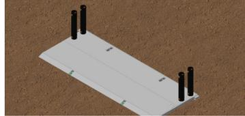
2) PLACE SPREADER PIPE ON TO COLLARS OR BRACKETS AND PIN IN PLACE. SECURE PINS WITH KEEPERS.
