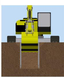
1) EXCAVATED TO GRADE JUST SLIGHTLY WIDER THAN THE TRENCH SHIELD. DIG WALLS VERTICAL TO MINIMUM OF 18" BELOW THE TOP OF THE SHIELD. SLOPE SOILS ABOVE SHIELD ACCORDING TO MANUFACTURER'S TABULATED DATA. INSTALL SHIELD IN TRENCH.
