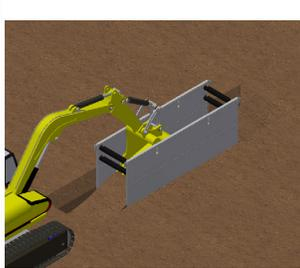
1) EXCAVATE UNTIL SOIL BEGINS TO CRUMBLE BEYOND DESIRED TRENCH WIDTH. PLACE SHIELD IN LINE OF EXCAVATION AND EXCAVATE FROM WITHIN.
