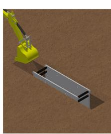
2) PERFORM DESIRED WORK, THEN EXCAVATE IN FRONT OF THE TRENCH SHIELD.
