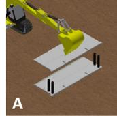
3A) LOWER SECOND SIDEWALL ONTO SPREADERS AND PIN IN PLACE.
