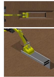
3) PULL SHIELD FORWARD BY FRONT TOP SPREADER PIPE OR PULLING EYES. PULLING EYES SHALL BE USED WITH SPREADERS WIDER THAN 72" OR WHEN SOIL PRESSURE IS SEVERE ENOUGH TO CAUSE SPREADER TO DEFLECT. CONTINUE EXCAVATING AND PULL SHIELD FORWARD, BACKFILL AS WORK PROGRESSES.
